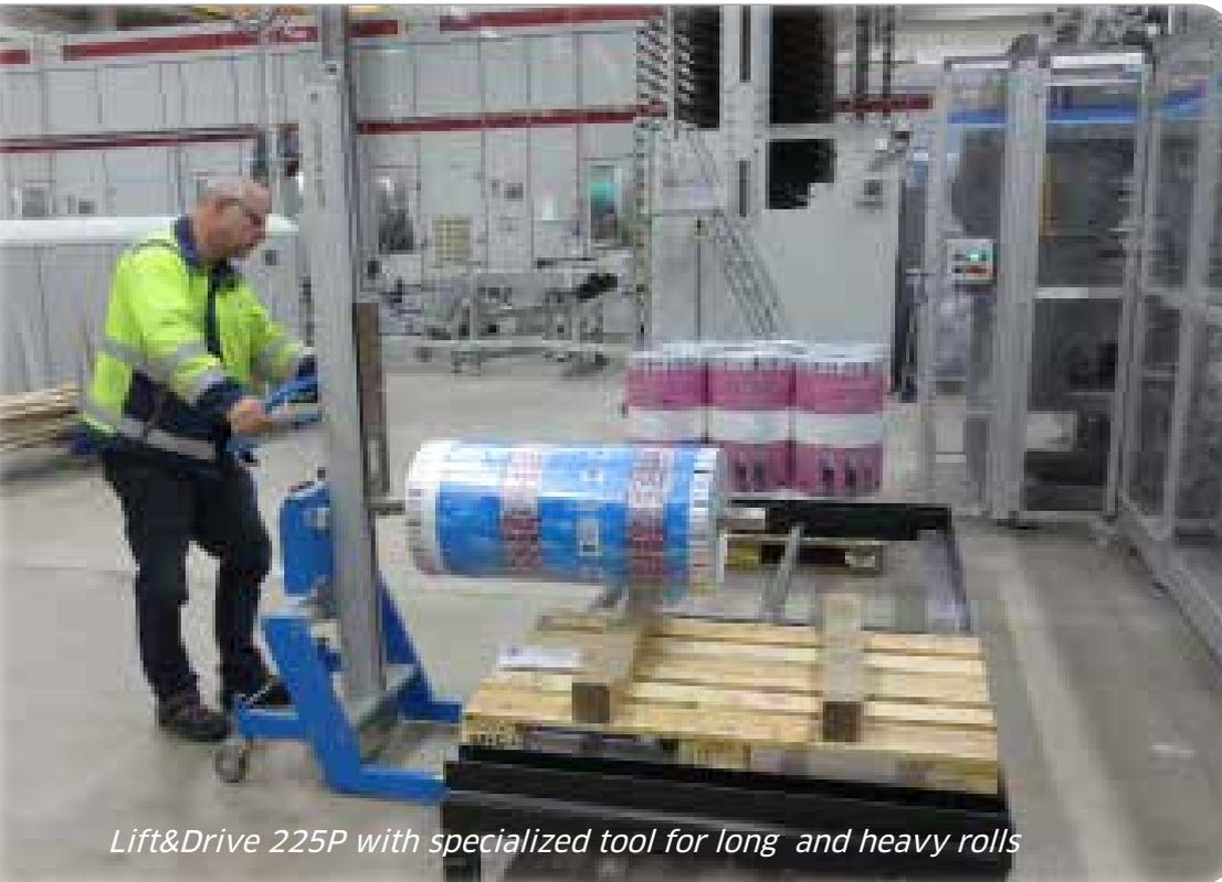
Lift&Drive 225P with specialized tool for long and heavy rolls
